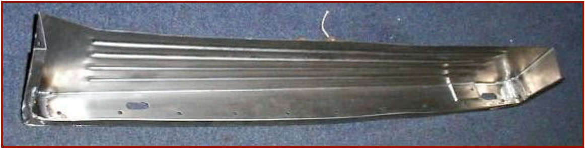
Lower Inner Door Frame Repair Panel – Top View Replaces Entire Door Bottom to 1” above the Hinge Mount
