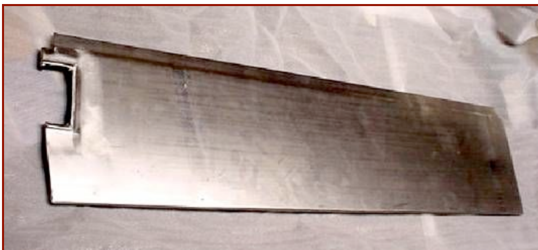
Lower Outer Door Panel Repair Section
